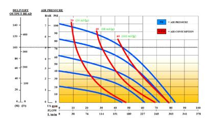
AIR PRESSURE: Tested at 100 psi / 690 kPa (not to exceed 125 psi / 861 kPa) FLOW RATE: 0 - 130 gpm / 300 Lpm FLUID CONNECTION: 2" / 50mm (Internal Thread) AIR INLET PORT: 1/2" / 15mm (Internal Thread) 3/4" / 19mm (Internal Thread) **EXHAUST PORT: DELIVERY PRESSURE:** Tested to 145psi / 1,000 kPa **SUCTION LIFT:** Tested to 24' / 7m dry and 30.5' / 9m wet **SOLIDS HANDLING:** 1.8" / 46mm PUMP WEIGHT: Yellow Series - 101 lbs / 45.8kg Red (FRAS) Series - 1118 lbs / 53.5kg
