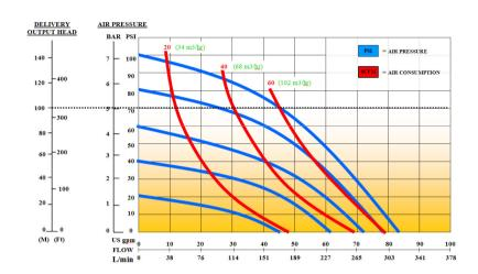
AIR PRESSURE: Tested at 100 psi / 690 kPa (not to exceed 125 psi / 861 kPa) FLOW RATE: 0 - 80 gpm / 300 Lpm FLUID CONNECTION: 2" / 50mm (Internal Thread) AIR INLET PORT: 1/2" / 15mm (Internal Thread) **EXHAUST PORT:** 3/4" / 19mm (Internal Thread) **DELIVERY PRESSURE:** Tested to 145 psi /1,000 kPa SUCTION LIFT: Tested to 19' / 6m dry and 31' / 9m wet SOLIDS HANDLING: .71" / 18mm PUMP WEIGHT: Yellow Series - 109 lbs / 49.4 kg Red (FRAS) Series - 128 lbs / 58.1kg
