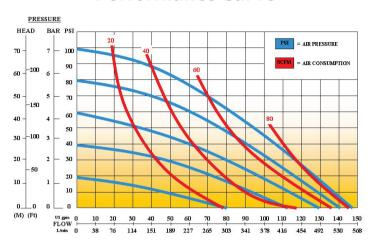
AIR PRESSURE: Tested at 100 psi / 690 kPa (not to exceed 125 psi / 861 kPa) FLOW RATE: 0-146 gpm / 553 Lpm FLUID CONNECTION: 2" / 50mm (Internal Thread) AIR INLET PORT: 1/2" / 15mm (Internal Thread) **EXHAUST PORT:** 3/4" / 19mm (Internal Thread) **DELIVERY PRESSURE:** Tested to 87 psi / 600 kPa SUCTION LIFT: Tested to 24' / 7m dry and 30.5' / 9m wet **SOLIDS HANDLING:** 1.8" / 46mm PUMP WEIGHT: Yellow Series - 51lbs / 23.1kg Red (FRAS) Series - 60lbs / 27.2kg
