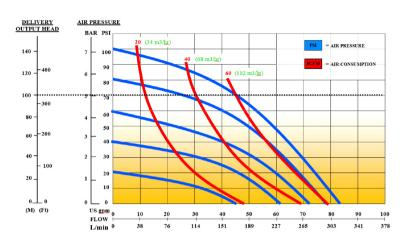
AIR PRESSURE: Tested at 100 psi / 690 kPa (not to exceed 125 psi / 861 kPa) FLOW RATE: 0 - 80 gpm / 300 Lpm FLUID CONNECTION: 2" / 50mm (Internal Thread) AIR INLET PORT: 1/2" / 15mm (Internal Thread) 3/4" / 19mm (Internal Thread) **EXHAUST PORT: DELIVERY PRESSURE:** Tested to 87 psi / 600 kPa **SUCTION LIFT:** Tested to 24' / 7m dry and 30.5' / 9m wet **SOLIDS HANDLING:** 1.8" / 46mm PUMP WEIGHT: Yellow Series - 101 lbs / 45.8kg
