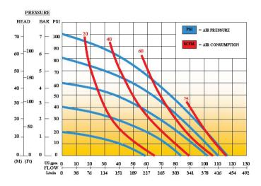
AIR PRESSURE: Tested at 100 psi / 690 kPa (not to exceed 125 psi / 861 kPa) FLOW RATE: 0-117 gpm / 443 Lpm FLUID CONNECTION: 1 1/2" / 40mm (Internal Thread) AIR INLET PORT: 1/2" / 15mm (Internal Thread) **EXHAUST PORT:** 3/4" / 19mm (Internal Thread) **DELIVERY PRESSURE:** Tested to 87 psi / 600 kPa SUCTION LIFT: Tested to 19' / 6m dry and 31' / 9m wet **SOLIDS HANDLING:** .55"/14mm PUMP WEIGHT: Yellow Series - 43 lbs / 19.5kg Red (FRAS) Series - 50 lbs / 22.7kg
