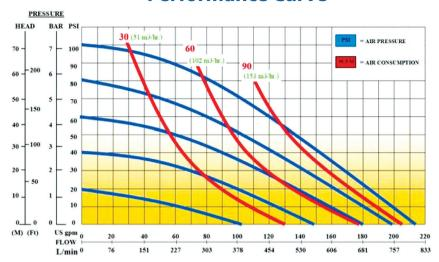
AIR PRESSURE: Tested at 100 psi / 690 kPa (not to exceed 125 psi / 861 kPa)
