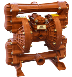
Red Series - P25SR FRAS (Fire Retardant Antistatic) Nylon Body- Hytel Elastomers- For Explosive Environment- ATEX M1 Rating
