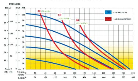
AIR PRESSURE: Tested at 100 psi / 690 kPa (not to exceed 125 psi / 861 kPa)
